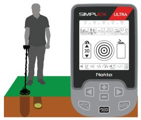
2) Keep the button pressed down and bring the search coil closer to the target slowly and parallel to the ground.
