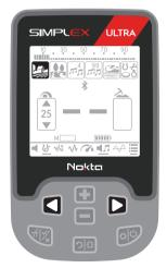
4) You can increase the sensitivity if needed. Increasing the sensitivity will offer you greater depth. However, if the surroundings or the ground cause excessive noise in the device, you need to lower the sensitivity setting.
