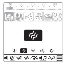
Vibration may not be felt in the All Metal mode with weak signals; it will be felt as the signal gets stronger. In other words, vibration does not start at the depth where the audio tones are heard but at a lesser depth. Therefore, if you are detecting with vibration only and audio tones are off, you can miss weaker and deeper signals.
