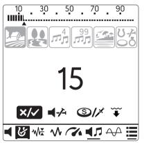
2. You can move the cursor using the plus (+) and minus (-) buttons and reject the ID you want by pressing the Ground Balance / Confirm button. Rejected IDs will be shown with lines over the ID scale.
