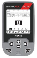
2. You can turn on or off the Bluetooth® connection using the plus (+) and minus (-) buttons. When it's off, the box will be displayed in white, when it's on, it will be in black.
