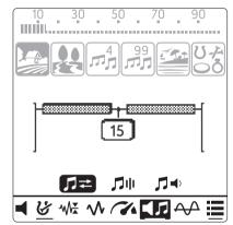
You can change the Tone Break point using the plus (+) and minus (-) buttons. To select the next zone, press the Ground Balance / Confirm button.
