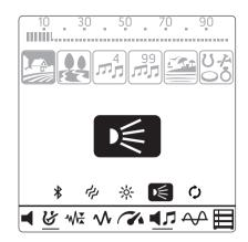
The LED Flashlight will always revert back to off position when the device is turned off and on again. This setting is common in all modes; change made in any mode also applies to the other modes.
