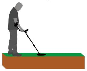
9) Since your device operates with the motion principle, swing the search coil right and left maintaining 5cm (2") distance above the ground. If the search coil does not move, the device will not provide any audio responses even if the coil is over a metal target.
