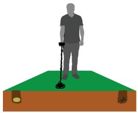
2. Press and hold down the Ground Balance / Confirm button and start pumping the search coil up and down from about 15–20 cm ( $\sim$ 6"– 8") above the ground down to 3 cm ( $\sim$ 1") off the ground with smooth movements and keeping it parallel to the ground.
