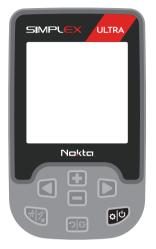
3) When the device is turned on, it will start in the 2-tone Field mode. You can change the mode based on ground conditions. For instance, if you are detecting on wet beach sand, you may want to select the Beach mode. You can find more details on search modes further in this manual.
