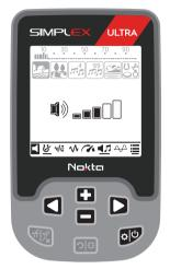
To exit the settings, press the Power & Settings button again. While in the settings menu, if no button is pressed for a while, settings will time out and the device will revert back to the main screen.
