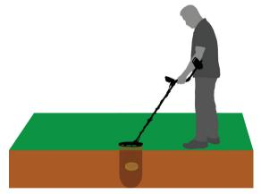
**NOTE:** Inexperienced users may put the search coil on the ground, press the pinpoint button and then scan over the target until they get experienced to perform the above pinpointing method.
