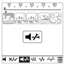
In the ULTRA version: After pressing the Power & Settings button, use the right and left buttons to select the Discrimination setting. Press the Ground Balance / Confirm button to access the upper settings. Using the right and left buttons, select the Iron Off setting which is the second setting. You can turn the iron on by using the plus (+) and minus (-) buttons.
