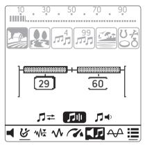
You can change the Tone Frequency using the plus (+) and minus (-) buttons. To select the next zone, press the Ground Balance / Confirm button.
