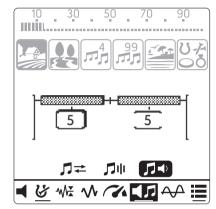
You can change the Tone Volume using the plus (+) and minus (-) buttons. To select the next zone, press the Ground Balance / Confirm button.
