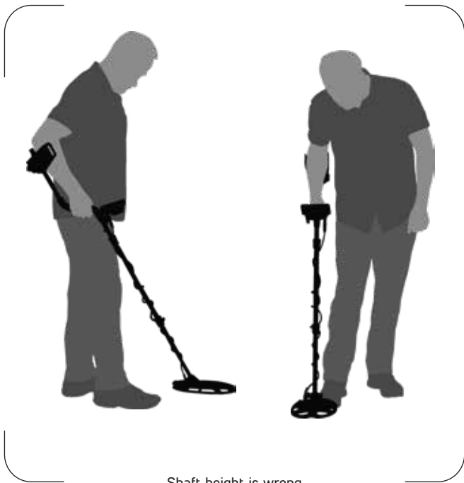
Shaft height is wrong
