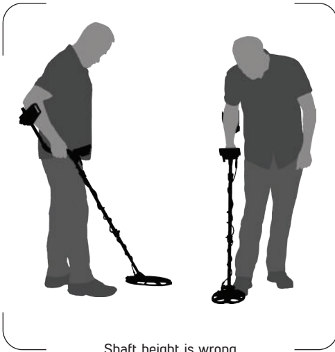
Shaft height is wrong
