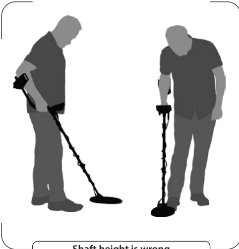
Shaft height is wrong
